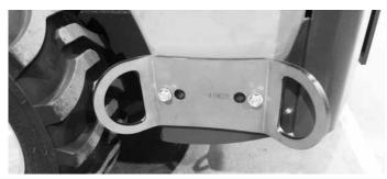
Tie down bracket A418623 installed at the side of rear frame. For side installation, two brackets are needed.
